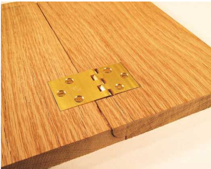
▲ Pic.3 The underside of the closed joint showing the hinge and screw positions
